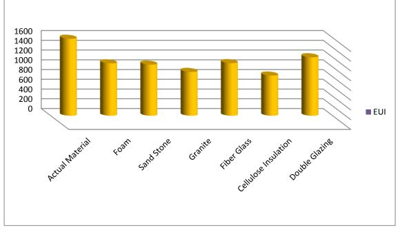
Figure 9. – The effect of alternatives on the energy consumption.
